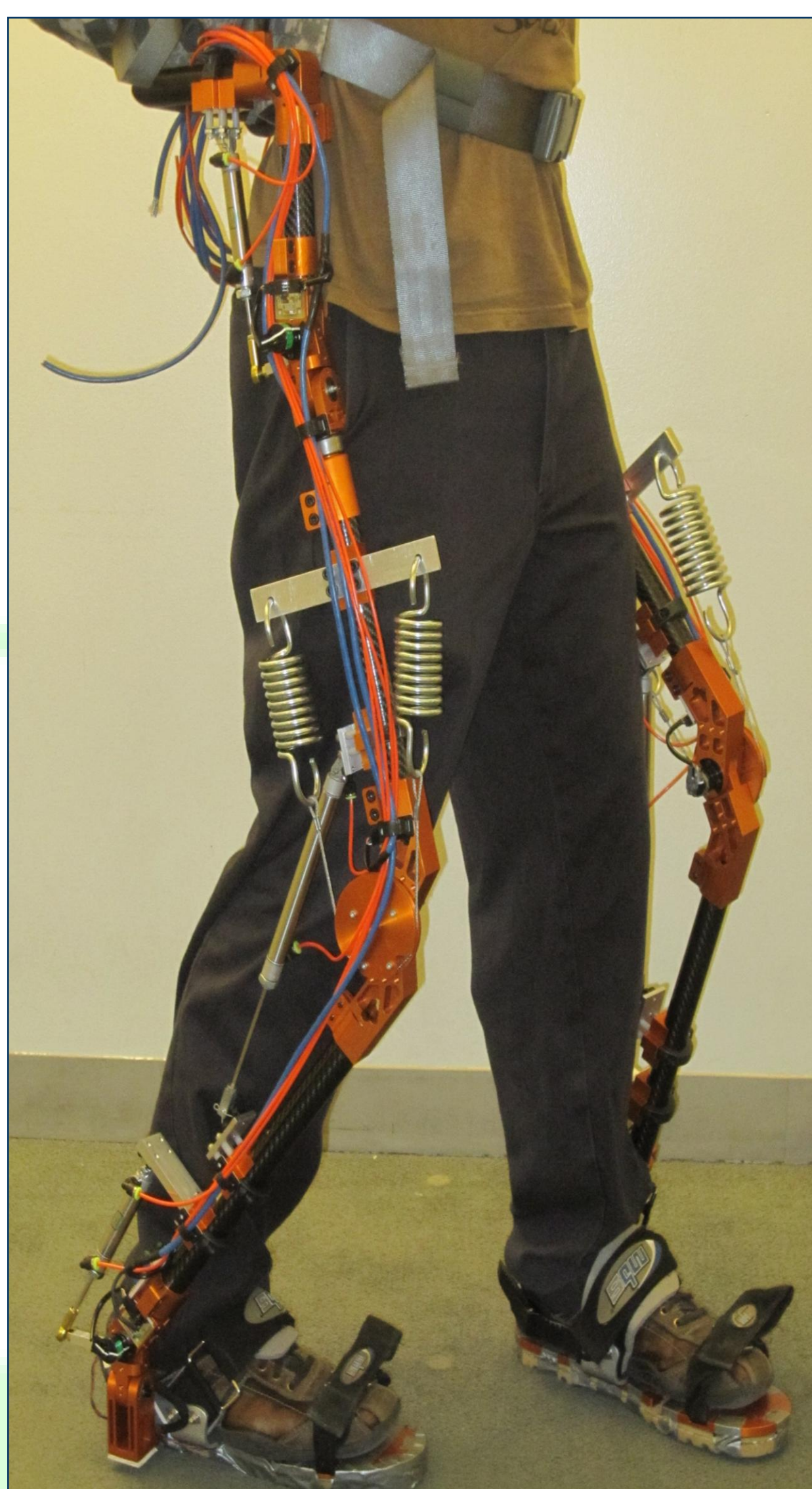
Figure 1. Mechanical movement of the piston cylinder assembly being fully compressed from a small knee bend.
